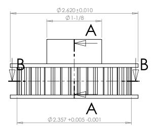
**NOTE: CORED PULLEYS** HAVE 1/16" THICK RIBS, REINFORCEMENT
